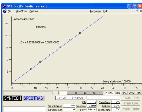
Six point calibration test up to 20 ppb
