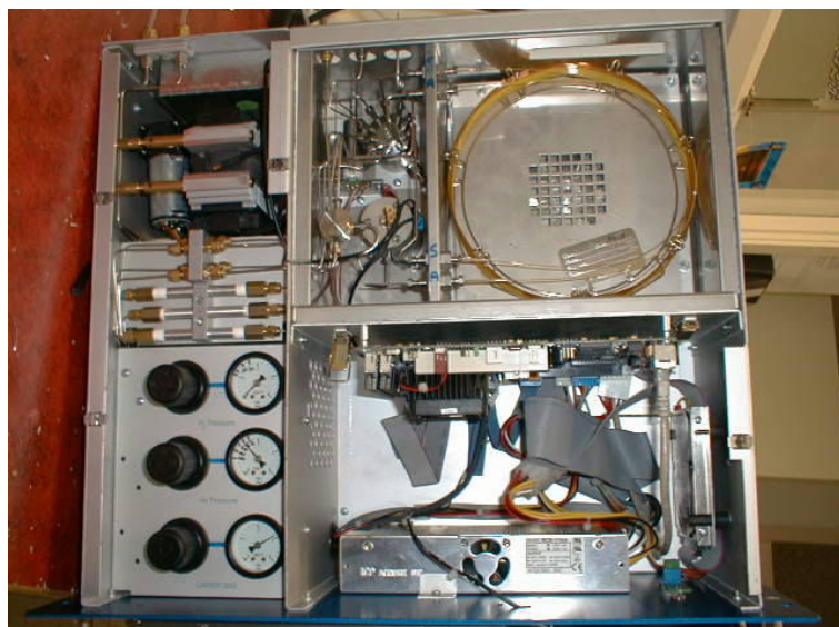
Gas chromatograph opened with oven at the right top. Still missing; (Photo of the small oven and photo of the double column in it)
