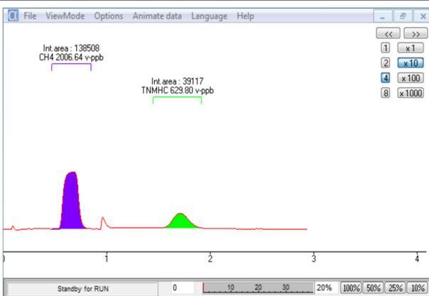
Measurement of ambient air with an Alpha 115
